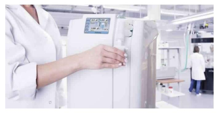
The Aquinity<sup>2</sup> P10 ultrapure water system is equipped with a reverse osmosis (RO) cell to produce deionised water directly into an integrated 10l tank.
