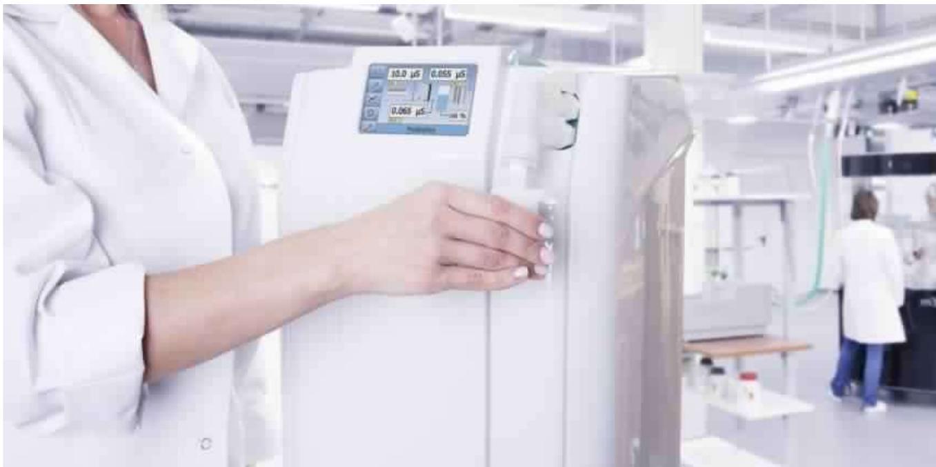
The Aquinity<sup>2</sup> P10 ultrapure water system is equipped with a reverse osmosis (RO) cell to produce deionised water directly into an integrated 10l tank.
